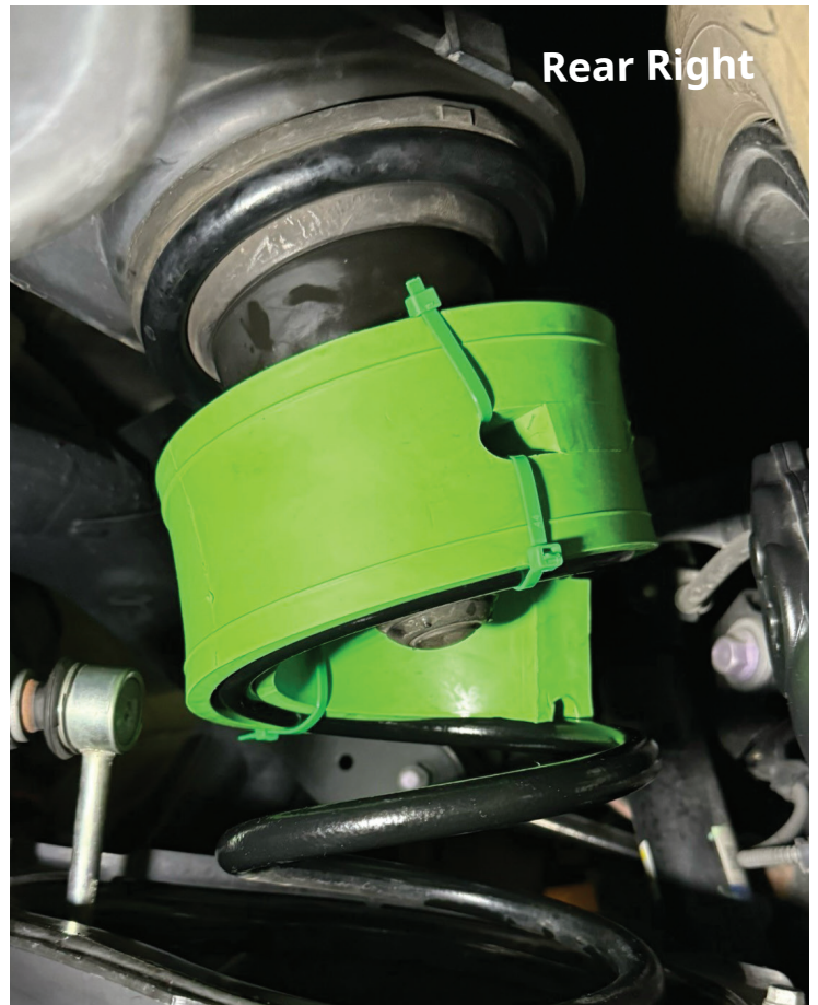
Ground Lifting Height : +0.5"
